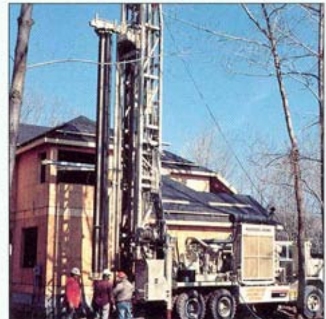
T4W Drillmaster rig is known around the world for drilling speed and reliability. Rotary or downhole drilling, plenty of on-board air power. Float-mounted deck power pack.
