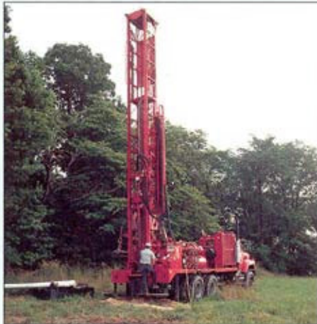
TH-55 Cyclone® is medium-weight rig with features you'd expect on larger machines. Tophead drive; 26,500-lb. (12,020-kg) pullback; I-R 600-cfm (17 m³/min.) air compressor.
